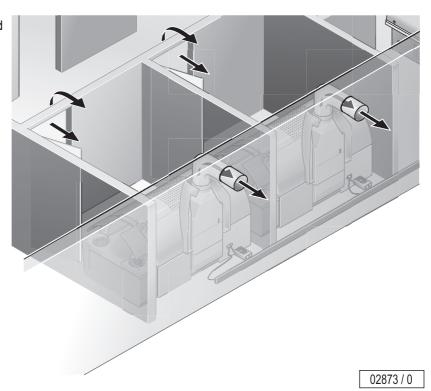
Inlet and exhaust air connection via a hanging studio ceiling with a separate exhaust air ducting
